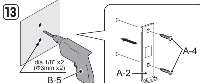
When mounting on a plaster board or tiled wall.
