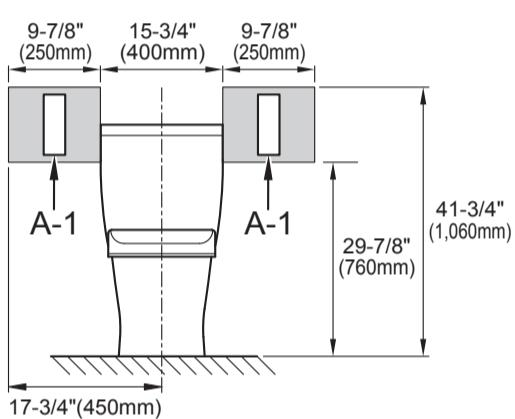
**12** Temporarily place the remote control in the position determined in **11** and confirm the signal reception of A-1.
